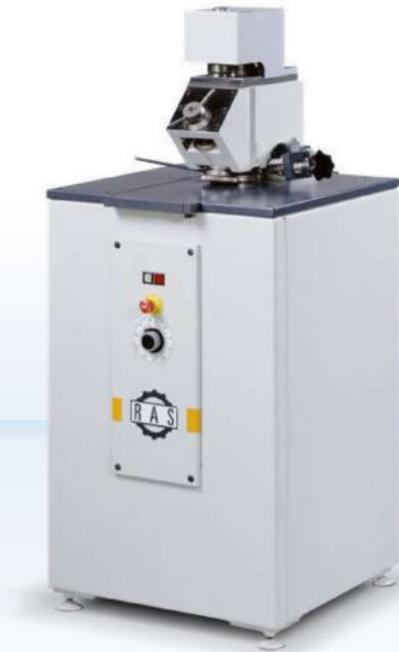
The RAS 21.20 flanging machine offer a proven technology in the ventilation industry, when arc segments are manufactured for air ducts. The forming rolls turns up 90 degree flanges on radius cheeks so that the parts are ready for Pittsburgh or Snaplock joints.
