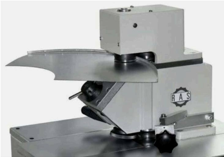
The forming rolls of the RAS flanging machine can create different flange heights—matching the required joints
