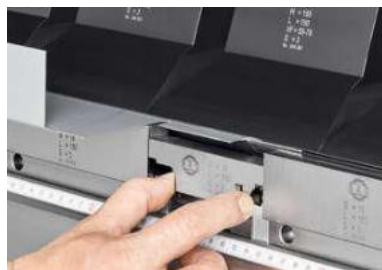
The DownTool in the folding beam can be simply lowered manually.
