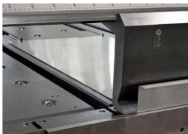
During the folding sequence the sheet rests on the machine table. No need to lift the part.
