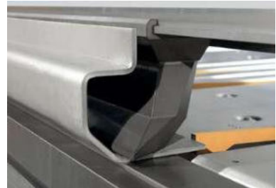
Upper beam tool with large front free space.
