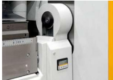
Optional digital display for folding beam adjustment.
