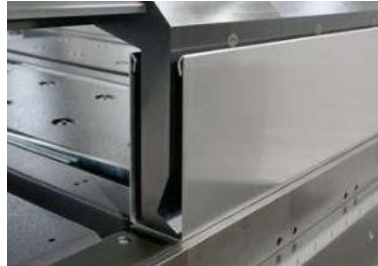
Part design flexibility due to slim but rigid tools.
