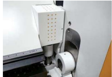
The PowerBooster clamps the blanks with 120 tons of pressure to guarantee straight bends.
