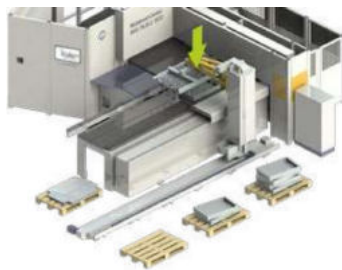
Picking up the bent part by the suction frame of the palletizer
