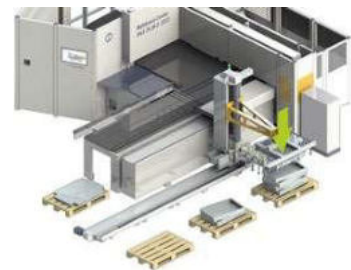
Horizontal stacking of a bent part on a pallet
