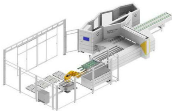
Multibend-Center with robot loading. Provision of the blanks on Euro-pallets. The robot can also flip the blanks. Intelligent robot: No programming or teaching required.
