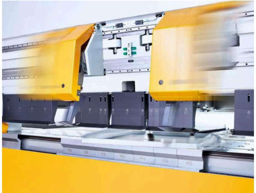
Fully automatic bending sequences: positioning, rotation, bending, and tool change.
