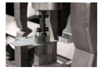
Several bending stations can be set up along the bending line. Complex bent parts are thus completed in one pass.
