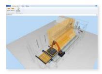
The generation of the optimal stacking routine of a finished part on the pallet is done by the RASpall program.
