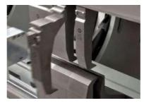
The automatic tool change allows quick part change and bending of small batches.
