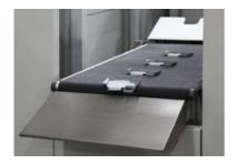
Bent parts that cannot be stacked can be discharged via the outfeed conveyor.
