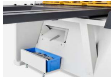
Small parts up to 200 x 500 mm can be delivered in a container in front of the machine.
