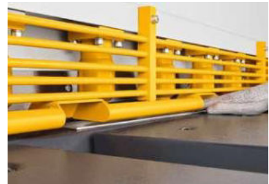
Deep finger pockets for best material utilization.
