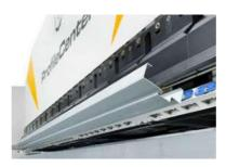
Complex part geometries can be bent due to the large free space around the tools.
