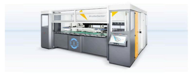
Flexible and automatic profile bends profiles such as door frames, window frames, elevator entries, electrical cabinet components or cable ducts in batch size 1. The unique FlexGripper handling system moves, rotates and flips the blank automatically during the bending process.
