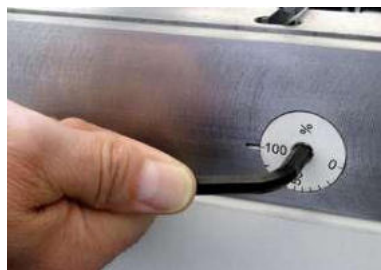
Setting the CrownTool (especially for step bending of radii).
