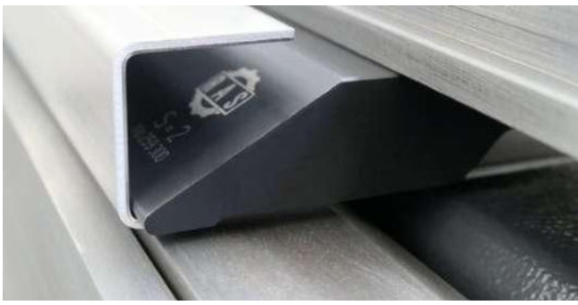
Tools with radius for bending aluminum.
