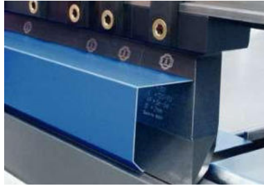
Segmented upper beam tools with front free space
