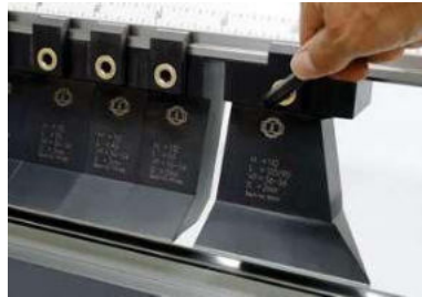
Tools with quick clamping system
