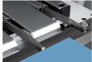
Stop finger at minimum stop dimension.
