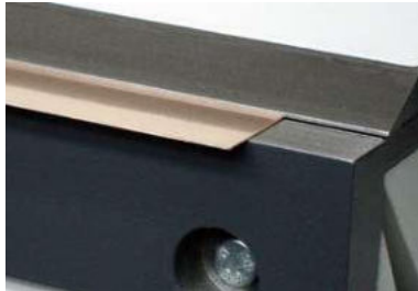
Automatic folding beam adjustment for thin and thick materials.
