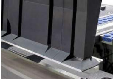
Only one set of upper cheek tools with heel to squeeze envelopes for great design flexibility. Bending of high four-sided parts.
