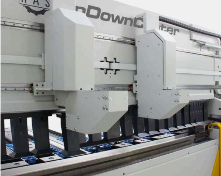
The automatic tool changer for quick tool set-ups extends production times.
