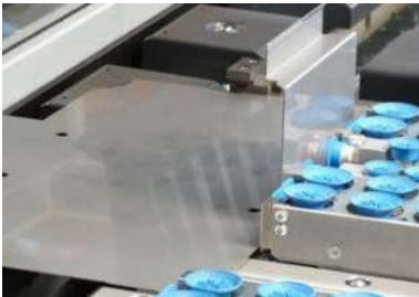
High flexibility in handling due to front suction cups and small part suction cups.
