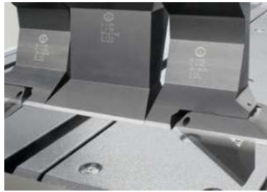
The SnapTool corner tools automatically retract from parts with side flanges.
