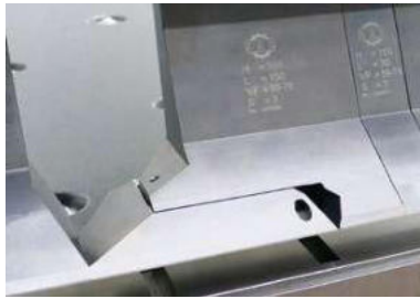
The SnapTool corner tools automatically retract from parts with side flanges.
