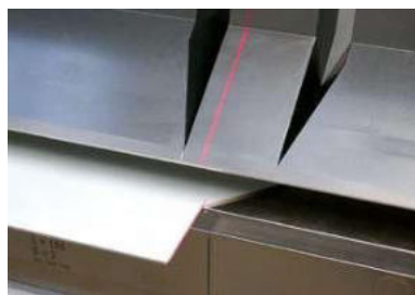
When working from the rear, the ViN also shows the blank loading position on the gauging system.
