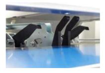
Secured bending accuracy due to automatic alignment of the blanks.
