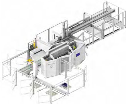
Multibend-Center with two station gantry loader and stacking with 3-Station Palletizer (max 11 stacks) or 5-Station Palletizer (max 15 stacks).
