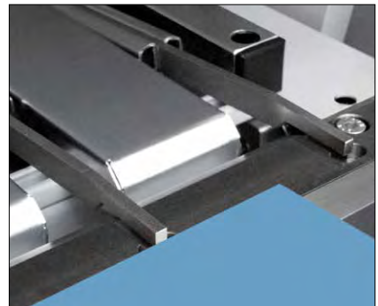
From min to max dimension in less than 2 seconds – fast and reliable backgauge finger adjustment.
