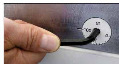
Setting the CrownTool (especially for step bending of radii).
