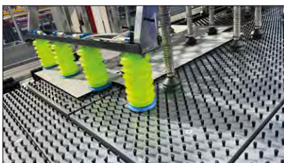
Loading system for automatic feeding of blanks from a stack of sheets with sorted and edge-precisely stacked sheets
