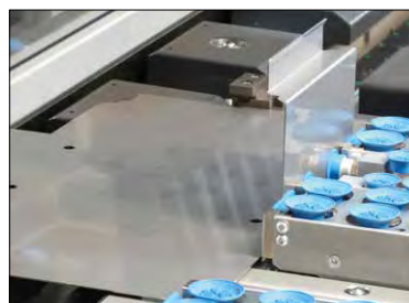
High flexibility in handling due to front suction cups and small part suction cups.
