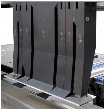
Only one set of upper cheek tools with heel to squeeze envelopes for great design flexibility. Bending of high four-sided parts.
