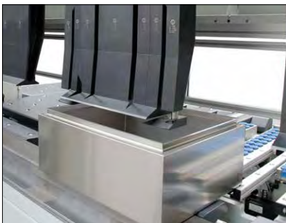
Upper beam tools for boxes up to 600 mm tall.
