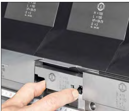
The DownTool in the folding beam can be simply lowered manually.
