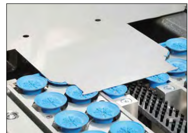
Suction cups for small parts allow safe positioning of small workpieces.
