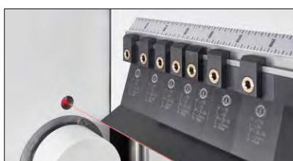
A laser automatically recognizes the exact tool height.
