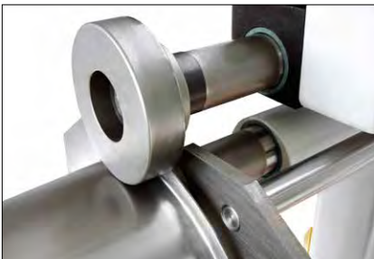
Flanging wheels FL: Flanging without swiveling the part.
