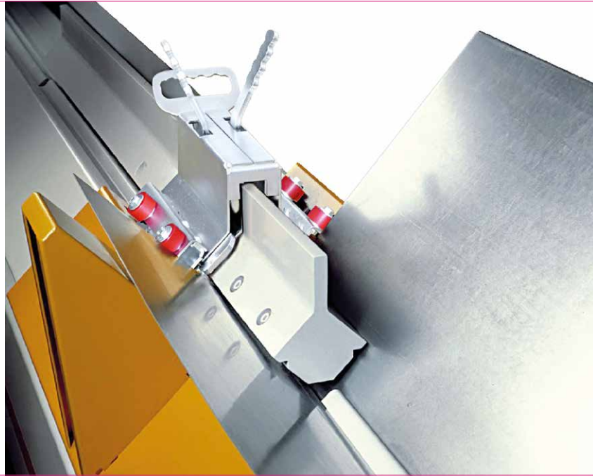
Autopilot and reinforced seaming bar on the RAS 20.12 DuctZipper.
