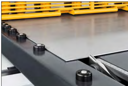
Front stops (available also with a precision scale) allow an accurate part positioning
