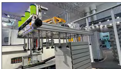
Loading system for automatic feeding of blanks from a stack of sheets with sorted and edge-precisely stacked sheets
