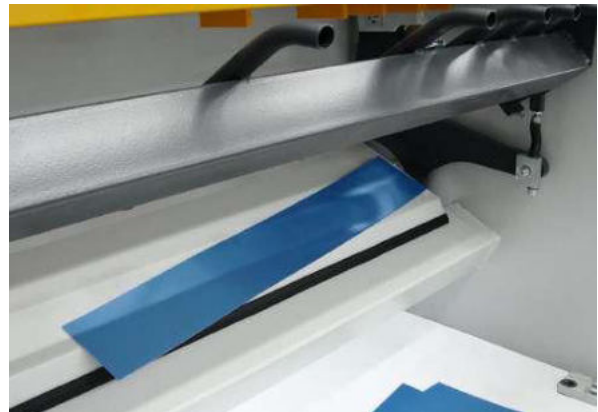
Parts chute for cut piece delivery to the rear.
